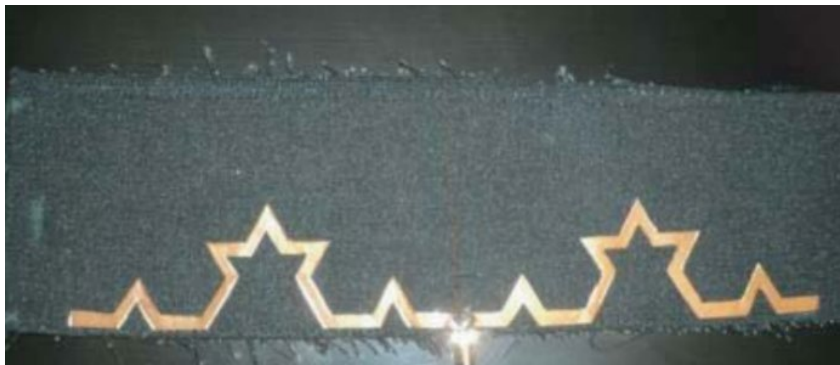
Figure 4. Fabricated photograph of the Koch fractal antenna on jeans cloth. Reproduced with permission from The Electromagnetics Academy under the terms of the Creative Commons Attribution 4.0 International License ( https://creativecommons.org/licenses/by/4.0/ ).
