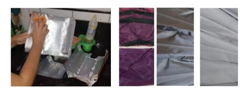
Figure 5.2. Tetra-Pak cardboard material preparation and umbrella fabric<sup>6</sup>
